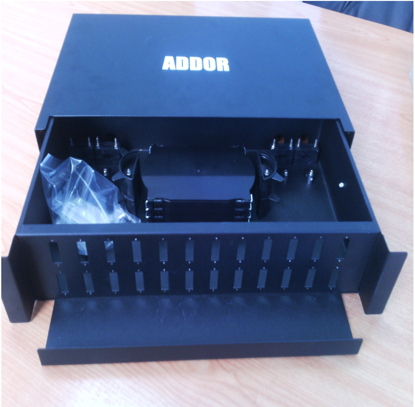
24 Port Patch Panel with splicing tray for SC duplex adaptor -
